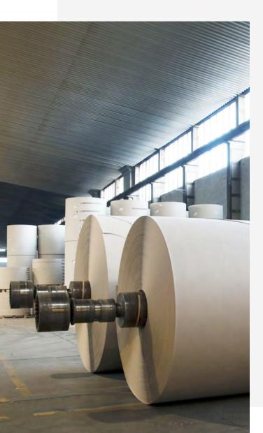
Paper type:Kraft linerboardSpeed:400-500 mpmBasis weight:170-195 g/m2Furnish:100% virgin unbleached Kraft
