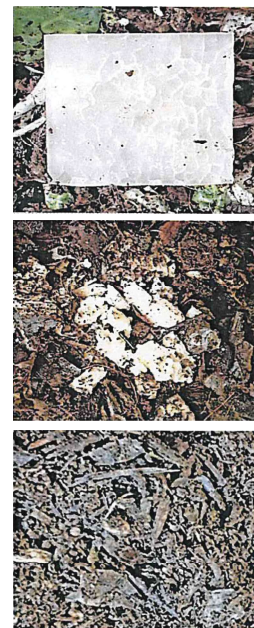
Figure 2. The appearance of TAPIOPLAST®TPS at (a) 0 day, (b) 7 days, and (c) 14 days, with the initial thickness of 3.39 mm (according to ISO 16929, disintegration test).
